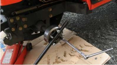
H. Get your socket & add Locktite to the studs on the spacer. Install the rim/wheel & now use the new Lock Washer & nuts from the spacer, making sure they are flip to the proper end. Torque the nuts to 110 ft. lbs for the rim in the same 3 steps as above.
