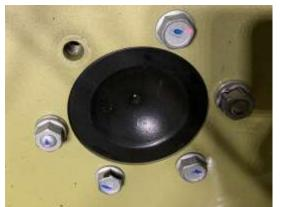
F.The factory bolts treads are 14 mmx1.5 tread, We have supplied new Lug bolt 14 mmx1.5 use these to install the spacer to the axle MImportant the OEM lug bolt are not long enough, do not ruese these.
