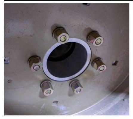
I. Check clearances around the Wheel, no point of contact should be noticed. Make sure to fully turn the steering left/right.
